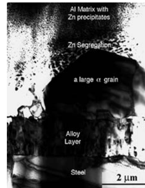
Figure 8 : Occurrence of \theta -FeAl 3 and \alpha -Fe 5 Si 2 Al 20 phases at 510°C strip preheat temperature and 80-250ms immersion time [10].
